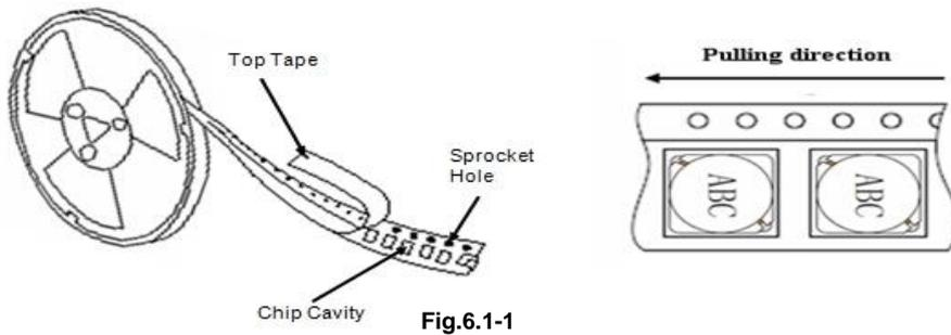
c. Reel and Taping Dimensions (Unit: mm)
