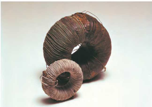
Figure 1 The First Ferrite Core in the World
