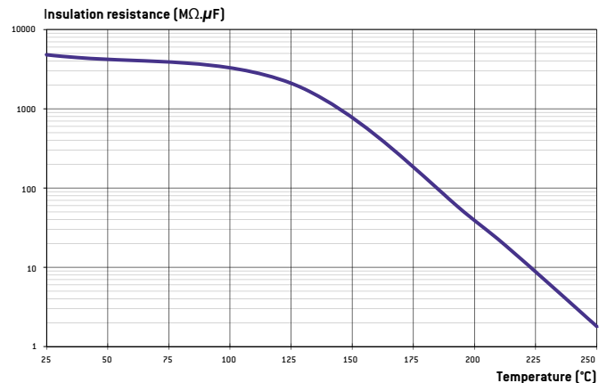
X7R: TYPICAL INSULATION RESISTANCE VERSUS TEMPERATURE
